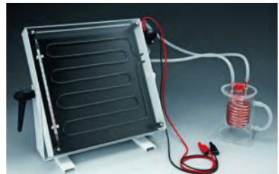
A Solar thermal collector Image by DJD Microtech is used under fair use https://www.djb.co.uk/ppen_solar_thermal_collector.htmlx
