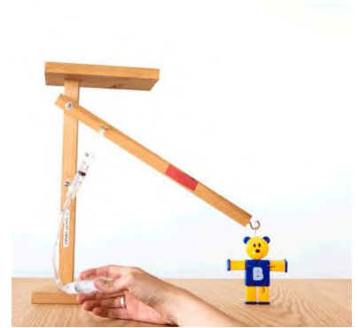
Image of a basic hydraulic powered articulated joint by Exploratorium is used under fair use https://www.exploratorium.edu/snacks/hydraulic-arm
