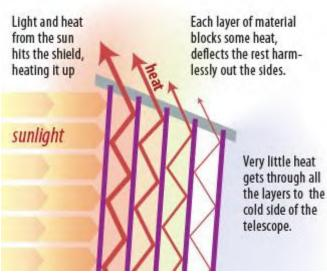
Illustration of the fiver layers of the sunshield and how each layer contributes to radiating away some of the Sun's heat. Image by STScl is used under fair use
