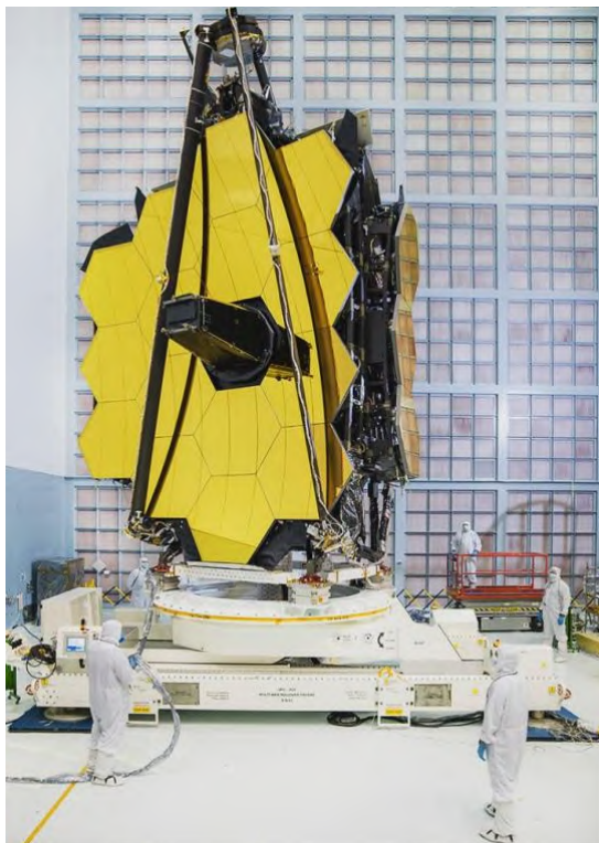
Folding wings of the Webb primary mirror
