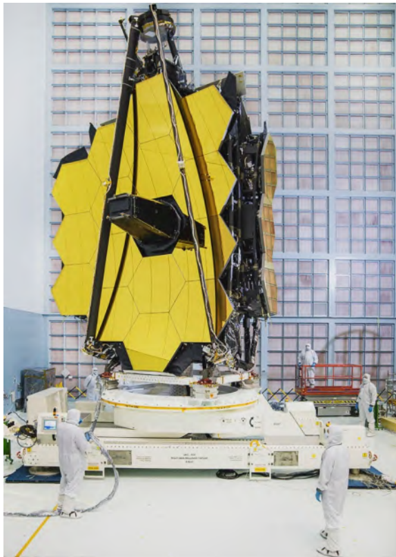
Folding wings of the Webb primary mirror Image by NASA, Chris Gunn used under fair use https://webb.nasa.gov/content/observatory/ote/mirrors/index.html#1b
