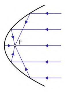
A diagram of a parabolic reflector, reflecting light rays to the focal point, F. Image by Filu released under a GNU Free Document license <a href="https://commons.wikimedia.org/wiki/File:Parabolic mirror-diagram.svg">https://commons.wikimedia.org/wiki/File:Parabolic mirror-diagram.svg</a>
