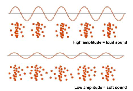
The distance between each successive compression or peak is called the wavelength. The shorter the wavelength, the more complete waves pass a given point each second. We measure how many waves pass per second as the frequency. One hertz (1 Hz) is one full wave per second.
