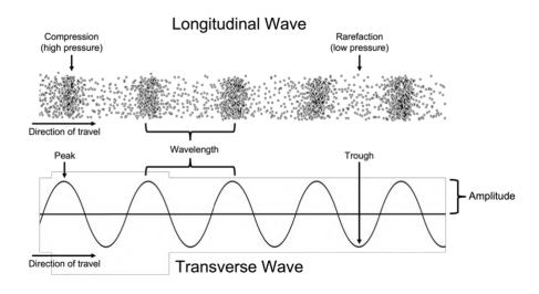
The more compressed the compressions, the greater the air pressure in these regions. We can model this as higher peaks (and lower troughs). We measure the height of the peaks as the **amplitude** of the wave. The greater the amplitude of a sound wave, the louder we hear it.
